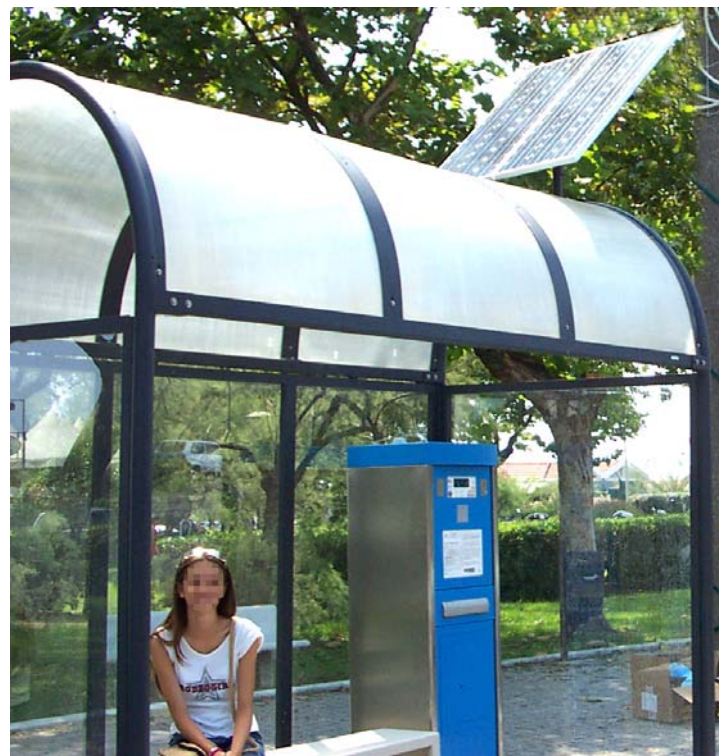
RTVM solare (CAT Carrara) - Sun powered RTVMs
