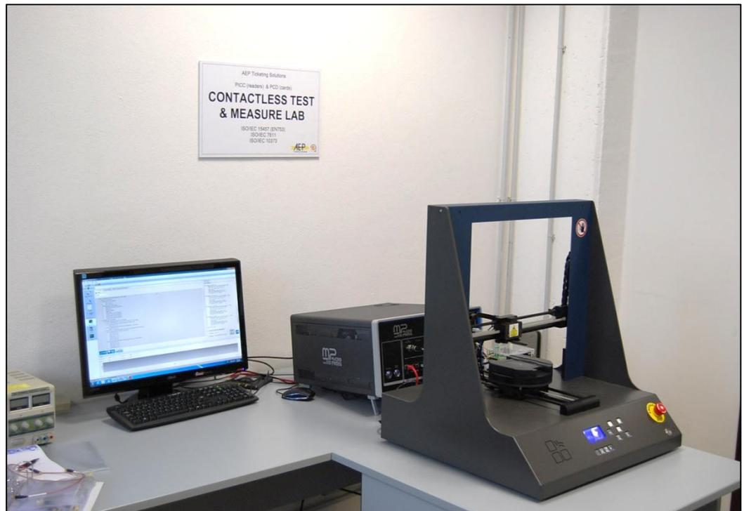
The Micropross MP300 with the 3-axis robot; used to verify readers and cards against the ISO IEC 14443-1, 2, 3 A & B and EMV ISO IEC 10373-6 standards.
