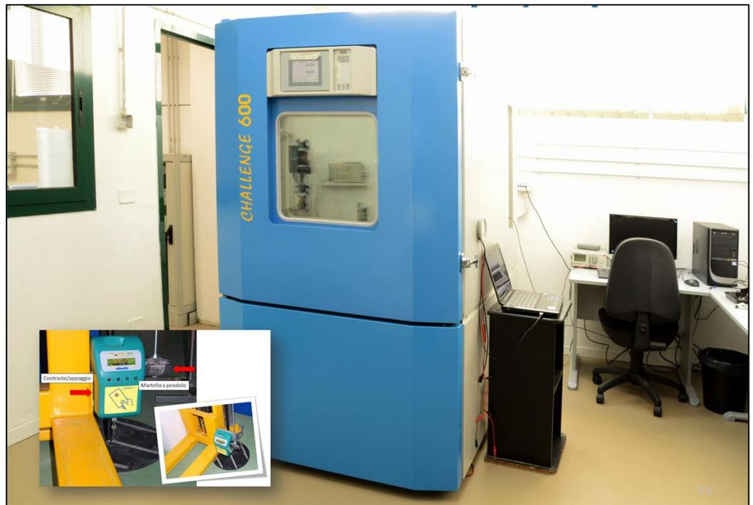
The temperature and humidity chamber which can carry out tests in conformity to many international standards such as the EN 60068-2 series. In the small frame, the hammer for the IK rating test as per EN 62262.
