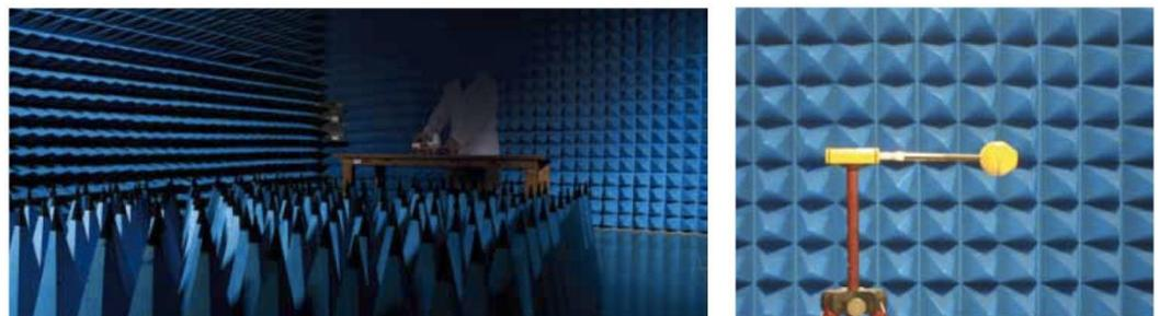
The semi-anechoic Cubit (9 x 8 x 7 m) room, certified to EN 50147-2, EN 50140, EN 60945, CISPR 16, ANSI C63.4, EN 61000 - 4 - 3 for the emission and immunity tests in the 30MHz - 18GHz band.
