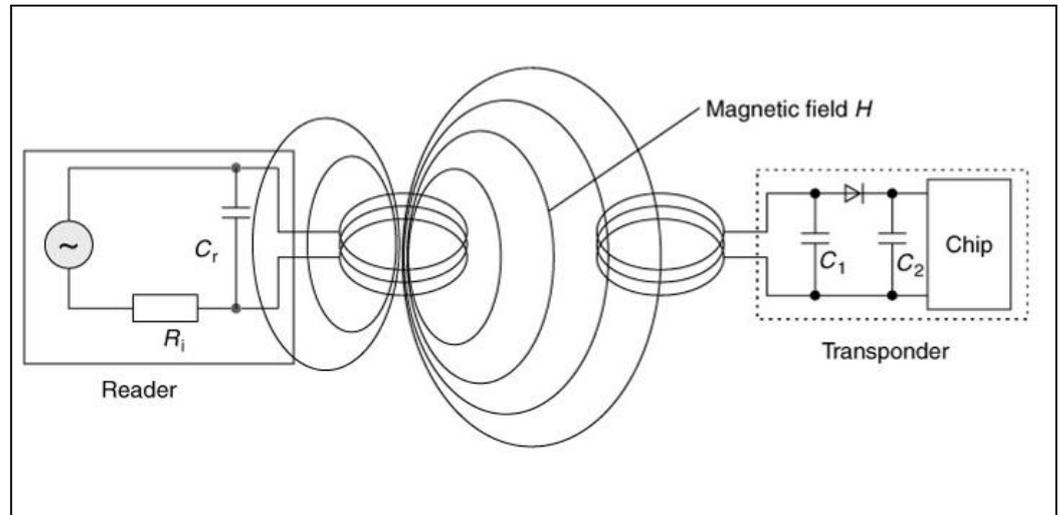
The smart cards communicate with the terminal through a radio frequency magnetic field (13,56 MHz) and are technically called PICC (Proximity Integrated Circuit Card).
