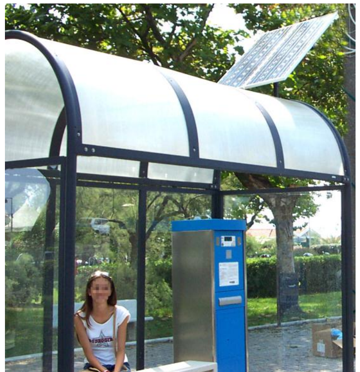
RTVM solare (CAT Carrara) - Sun powered RTVMs
